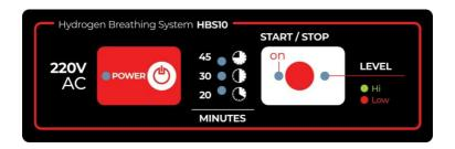
From the **POWER** button (white round button in the red rectangle) turn on the power to the device. When one of the **blue timer LEDs** lights up, power has been turned on.
